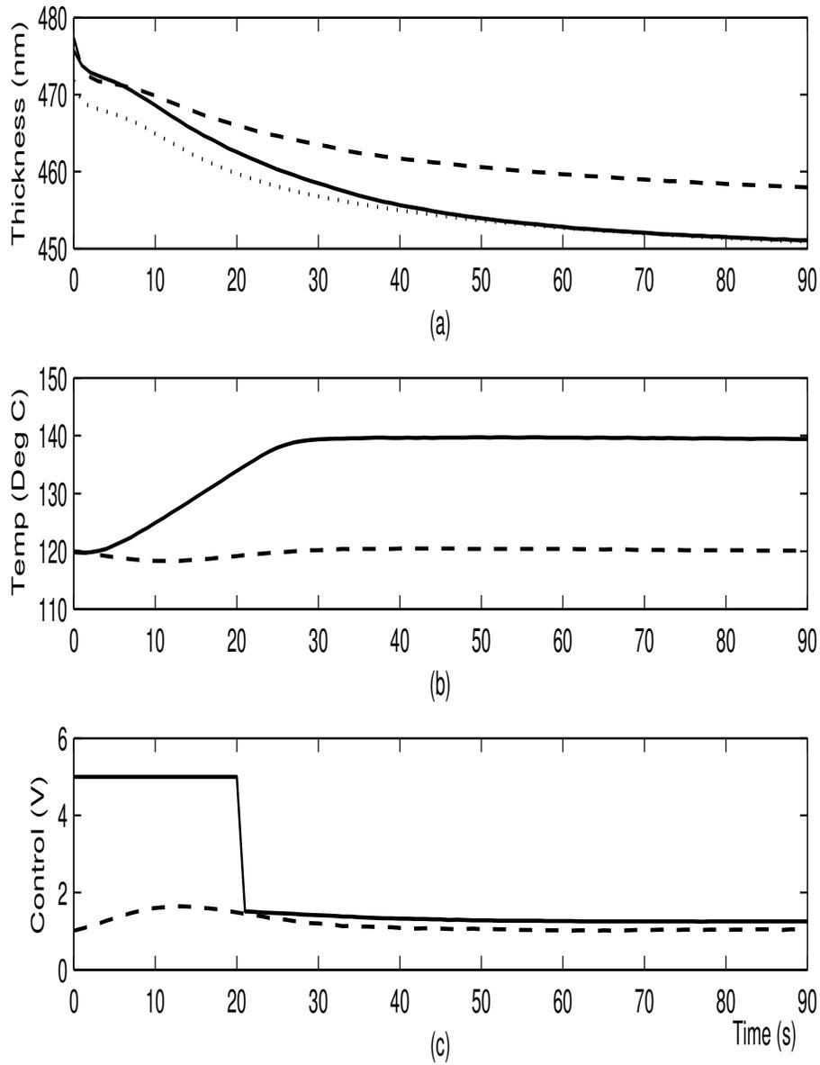
Fig. 3.4. Post-apply bake. (a) Photoresist thickness. (b) Bake plate temperature. (c) Control signal,  $u$ , in Voltage (V). Solid-line: Wafer 1; dashed-line: Wafer 5; dotted-line: desired photoresist thickness.
