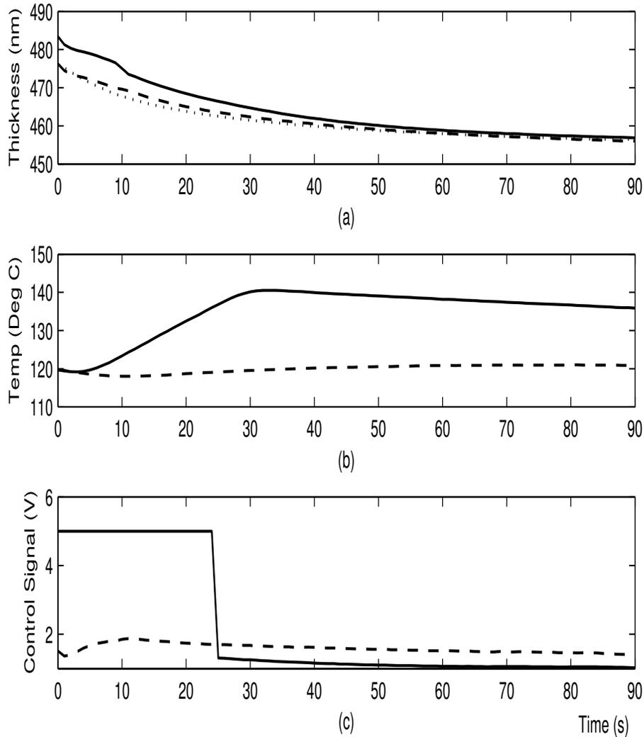
Fig. 3.8. Post-apply bake for Wafer 10 within-wafer CD control. (a) Photoresist thickness; (b) Bake plate temperature; (c) Control signal,  $u$ , in Voltage (V). Solid-line: near center of wafer; dashed-line: near edge of wafer; dotted-line: desired photoresist thickness.
