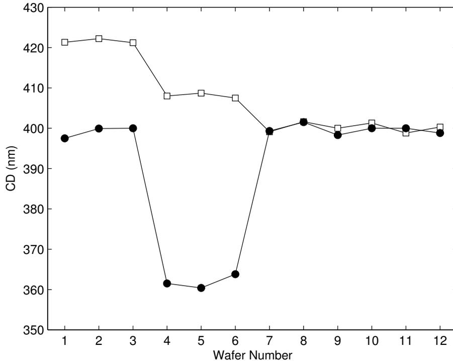
Fig. 2.4. Critical dimension measurements. Circle: center; Square: edge. Wafer 1–3: flat wafer with conventional baking; Wafer 4–6: warped wafer with conventional baking; Wafer 7–9: flat wafer with optimized baking; Wafer 10–12: warped wafer with real-time on-line adjustment of bake plate temperature setpoints.
