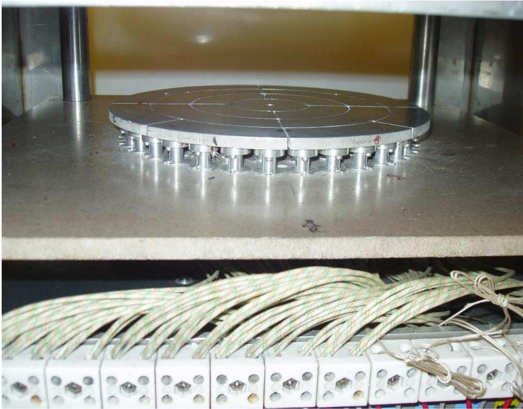
Fig. 4.3. Photograph of the multizone bake plate
