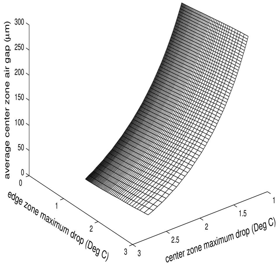
Fig. 2.7. Center-zone average air-gap versus bake plate maximum temperature drops.
