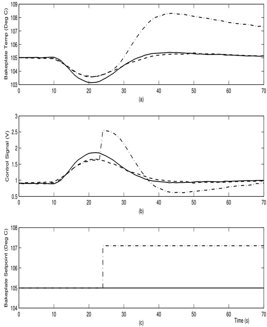
Fig. 1.3. Post-exposure bake temperature and power. Solid line: Flat Wafer; Dashed line: Warped wafer; Dash-dotted line: Warped wafer with setpoint adjustment.
