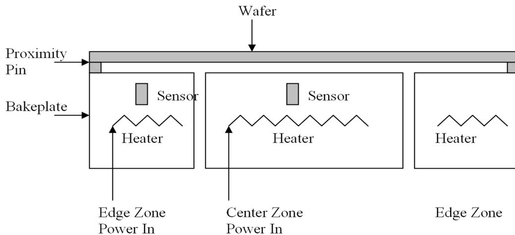
Fig. 3.9. Schematic diagram of a two-zone bake plate.
