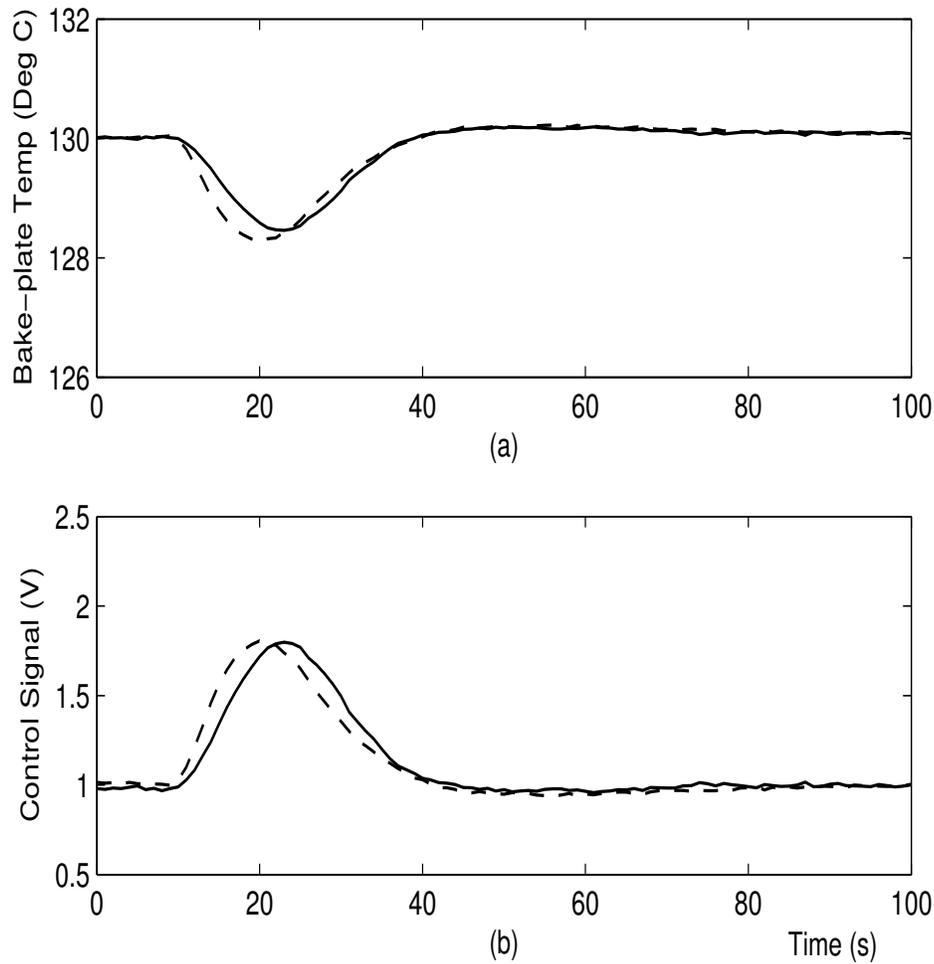
Fig. 2.2. Baking of Warped Wafer 4. Solid-line: center; Dashed-line: edge.
