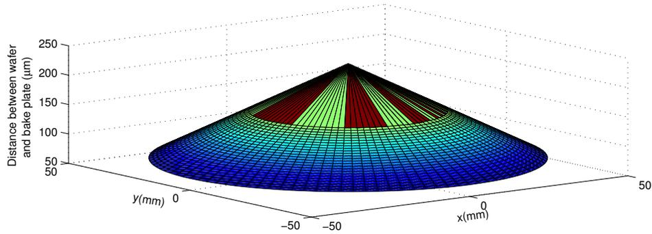
Fig. 2.10. Estimated profile of warped wafer 10
