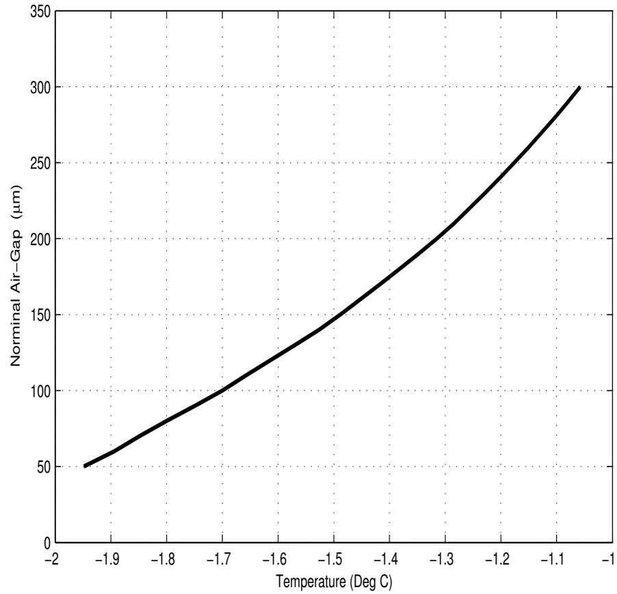
Fig. 2.12. Nominal air-gap,  $l_a$ , versus maximum temperature drop.
