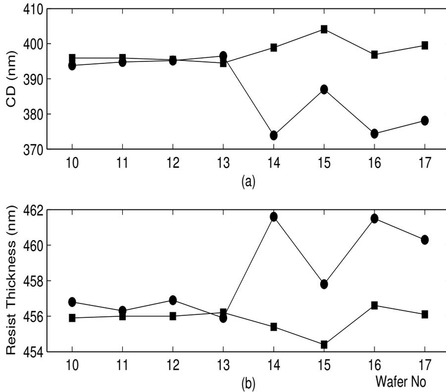
Fig. 3.6. Within-Wafer photoresist thickness and CD. Circle: near center of wafer; square: near edge of wafer.
