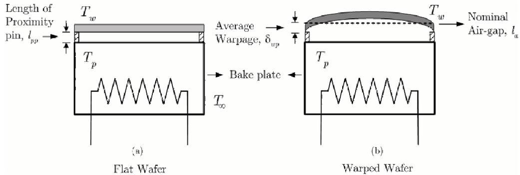
Fig. 1.2. Schematic diagram of the baking process.
