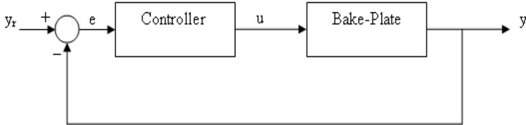
Fig. 3.3. Block diagram of the control system.
