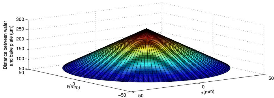
Fig. 2.11. Estimated profile of warped wafer 3
