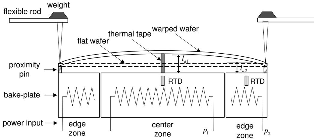
Fig. 2.3. Baking of Wafer.
