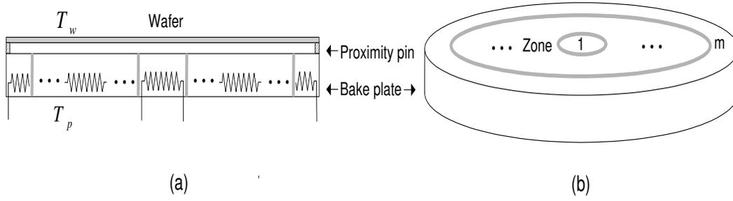
Fig. 4.2. Schematic Diagram of the multizone bake plate
