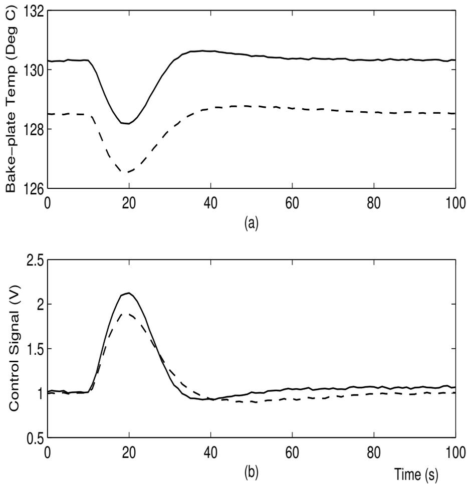
Fig. 2.6. Bake plate setpoint adjusted to give uniform CD for Flat Wafer 7. Solid-line: center; Dashed-line: edge.
