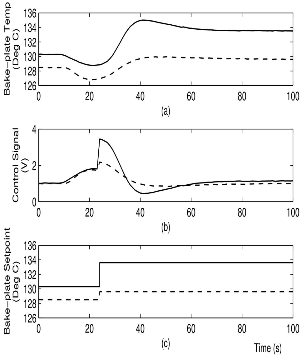
Fig. 2.9. Bake plate setpoints adjusted in real-time once warpage was detected to give uniform CD for Warped Wafer 10. Solid-line: center; Dashed-line: edge.
