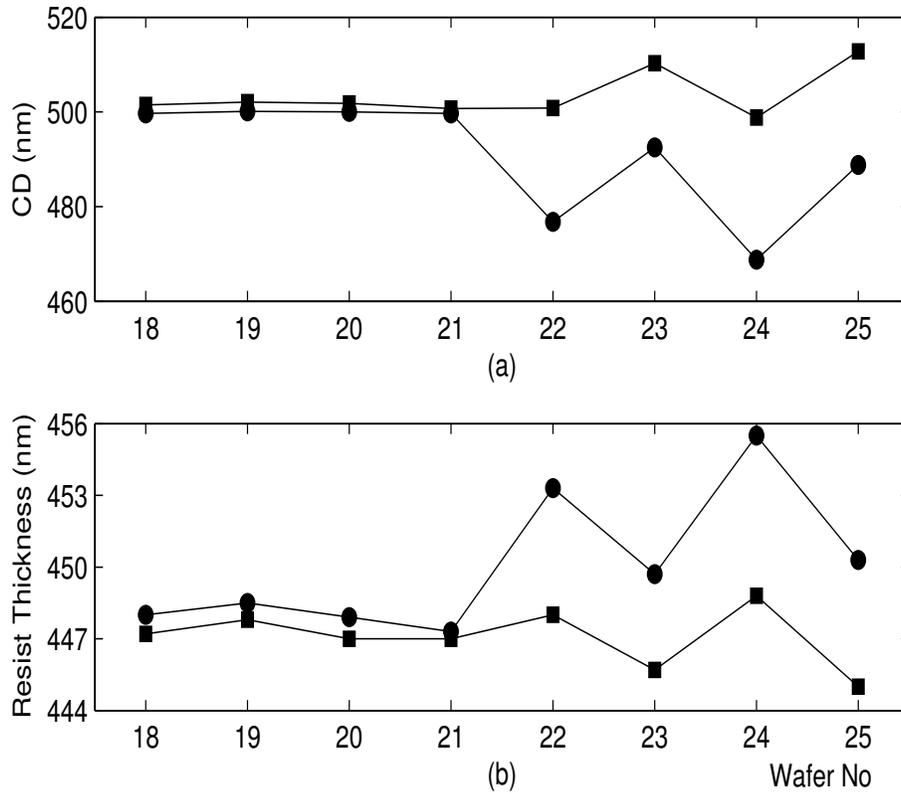
Fig. 3.7. Within-Wafer photoresist thickness and CD. Circle: near center of wafer; square: near edge of wafer.
