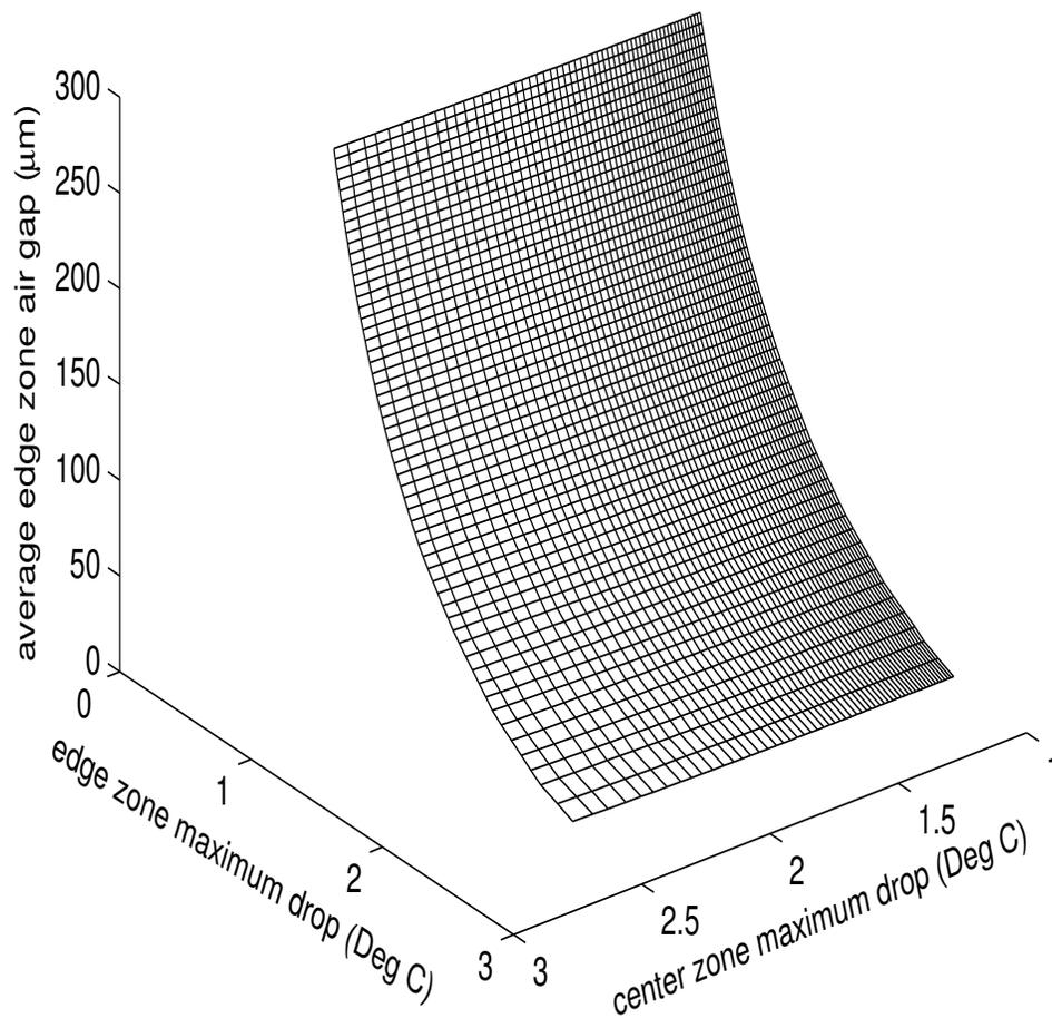
Fig. 2.8. Edge-zone average air-gap versus bake plate maximum temperature drops.
