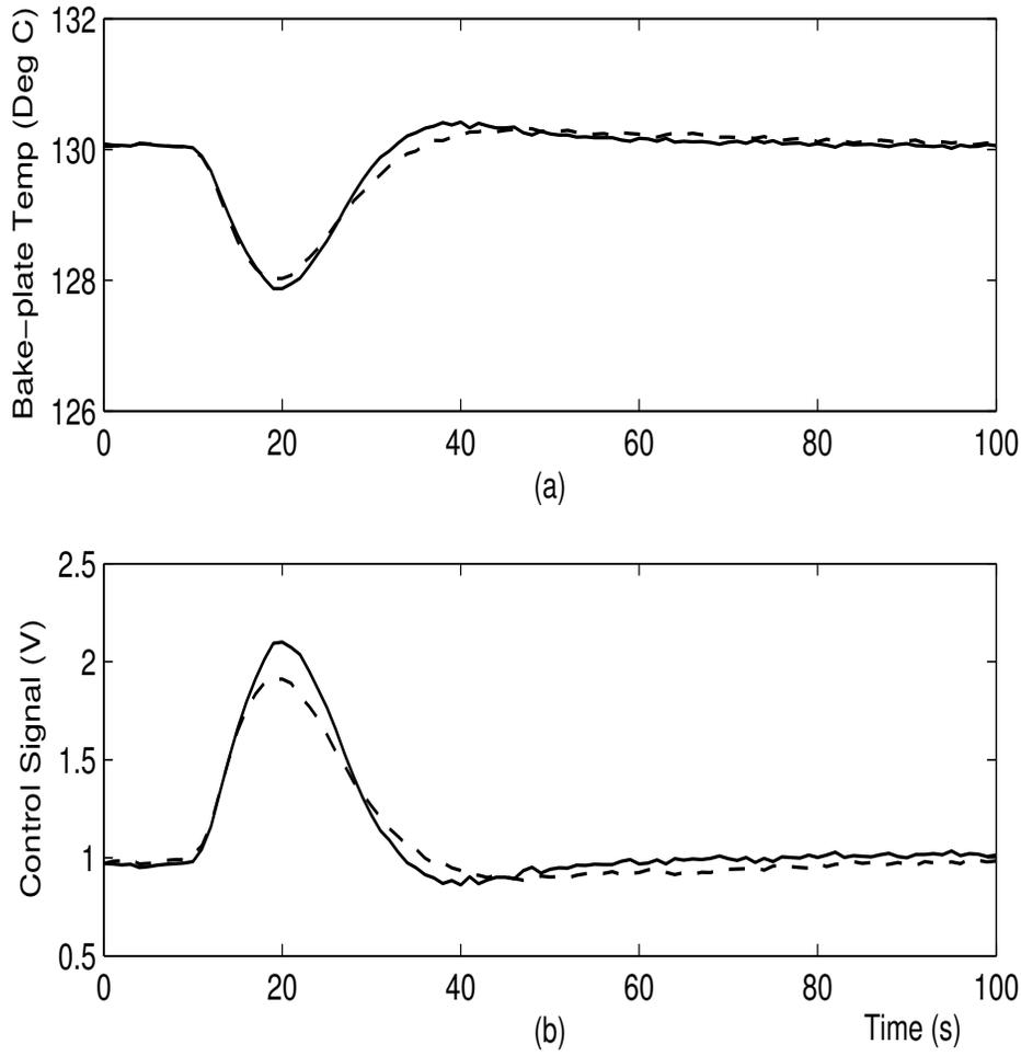
Fig. 2.1. Baking of Flat Wafer 1. Solid-line: center; Dashed-line: edge.
