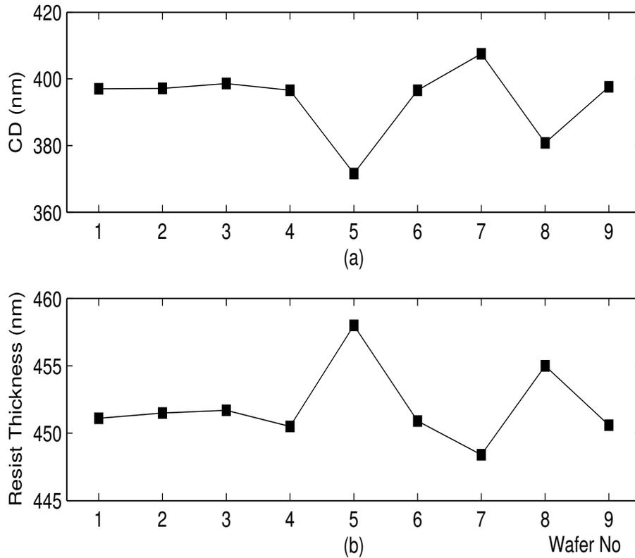
Fig. 3.5. Wafer-to-Wafer photoresist thickness and CD.
