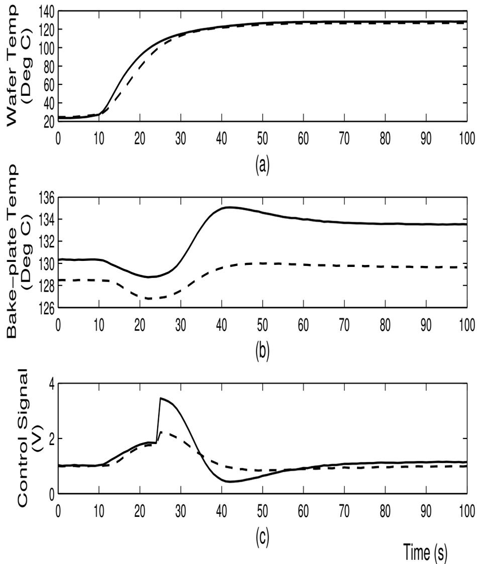
Fig. 2.5. Temperature measurement on a warped wafer with no photoresist nor pattern. Solid-line: center; Dashed-line: edge. The first plot shows the wafer temperature measured with RTDs. The second plot shows bake plate temperature where setpoint adjustments are made in the midway. The third plot shows the control signal.
