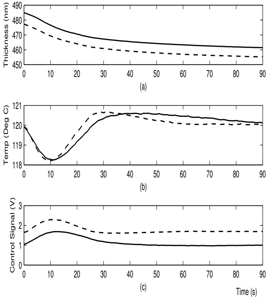
Fig. 3.10. Post-apply bake for Wafer 14 with no photoresist thickness control. (a) Photoresist thickness. (b) Bake plate temperature. (c) Control signal,  $u$ , in Voltage (V). Solid-line: near center of wafer; dashed-line: near edge of wafer.
