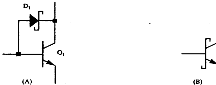
FIGURE 8.9 (A) Schottky-clamped NPN transistor and (B) its conventional schematic symbol.
