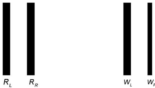
Figure 4.8 Lines of equal width ( R_L = R_R ) on the reticle print with different widths ( W_L \neq W_R ) on the wafer in the presence of coma.
